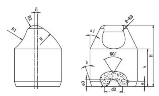
We produce Button bits in tungsten carbide with various types. Carbide buttons are widely used in oil filed drilling, because of its high strength and good wear resistance. Based on the different functions, the carbide buttons has been divided into many styles, and they often applied in roller cone bits, geotechnical drilling tools, DTH bits and
